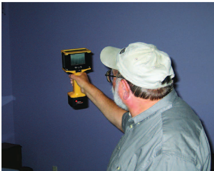
Infrared cameras can help energy auditors pinpoint areas of air loss. Source: Polk-Burnett Electric Cooperative
